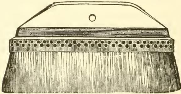
Fig. 15. Roofing Brush.
