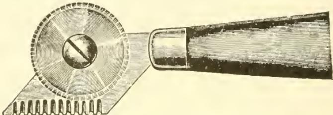
Fig. 59. Combination Casing and Corner Knife.
