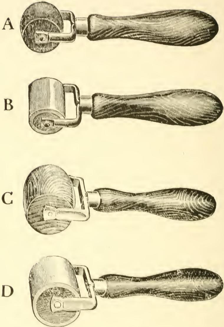
Fig. 50. Paperhanger's Seam Rollers.
